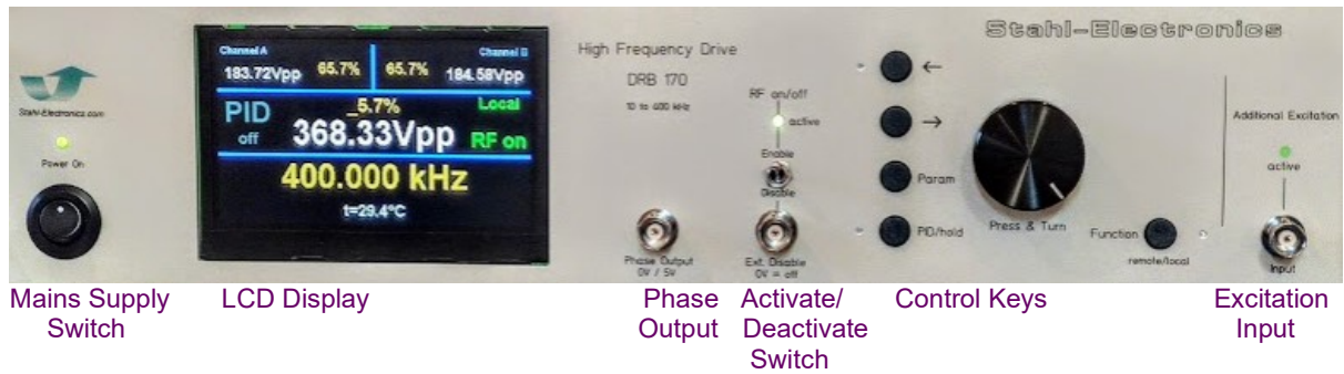
Fig. 3a The front plate contains the main control elements of the device:
