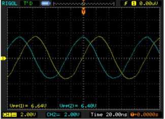
A2: Typical output waveform at 10MHz (Quad 1-10), 6.4Vpp output voltage, ch. B and C
