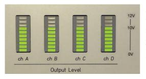
into the red range means bringing the output amplifiers to higher voltages while slowly going into saturation. This is a "smooth" and not a sudden process, which means that a slight overdrive at outputs might be still acceptable.
