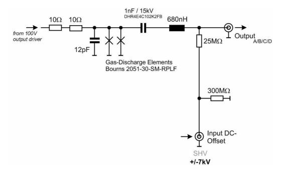
fig. A13: Circuit diagram of high voltage offset output stage +/-7kV floating version. An external DC offset of up to +/-7kV may be applied and is superposed to the AC signals from the internal phase shifter by means of a simple RC circuitry. Diagram shows one of four branches.
