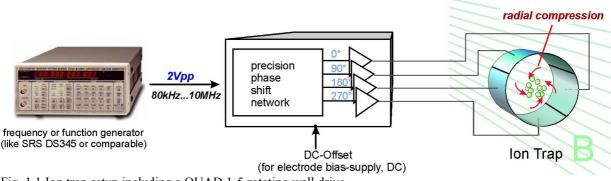
Fig. 1.1 Ion trap setup including a QUAD 1-5 rotating wall drive
