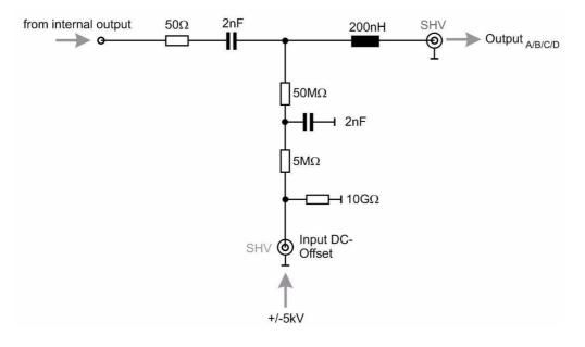
fig. A12: Circuit diagram of high voltage offset output stage. An externally supplied DC offset of up to  $\pm/-5$ kV (max. value depends on rating) is filtered by a 5M $\Omega$  x 2nF low pass and subsequently superposed to the AC signals from the internal phase shifter. Diagram shows one of four branches.
