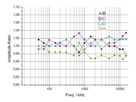
fig. A11: Typical amplitude mismatch vs. frequency Graph shows voltage ratios between output channels measurement device: oscilloscope TDS 210 (Tektronix)
