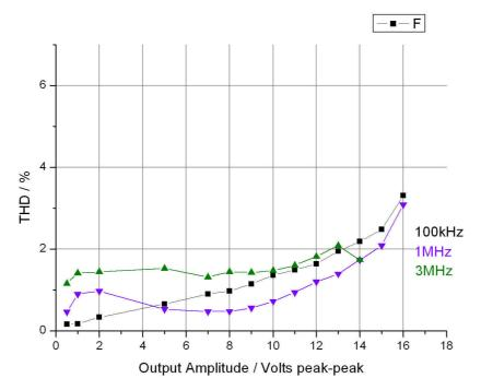
fig. A9: Non-linearity at high output levels (total harmonic distortion, THD), 10Vpp version load on output: 150pF // 10 MOhm, measurement device: Picoscope 3224
