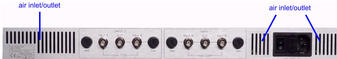
fig. 3.1: Keep air vents always cleared to ensure sufficient ventilation
