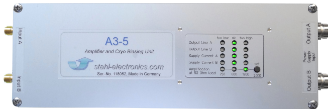
Figure 4: the roomtemperature controller indicates the status of the cryo amplifier and allows for setting the overall-amplification factor. The stated values of amplification factors refer to cryogenic operation and 50 Ohm termination at the roomtemperature controller outputs.
