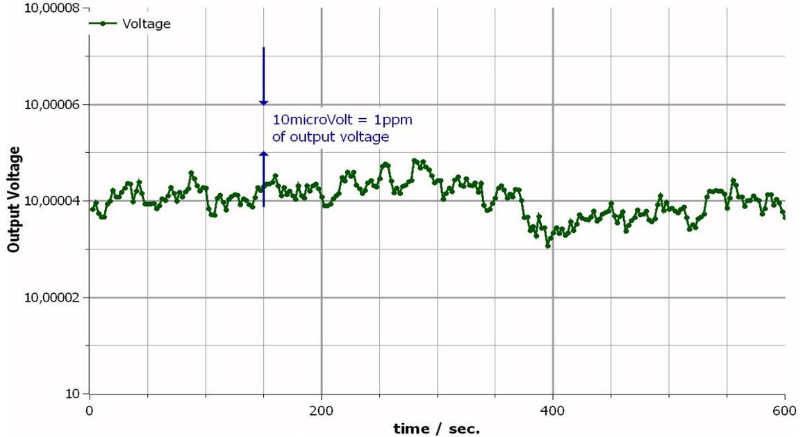
This figure illustrates the typical stability of an output channel at +10V, BSA series, over a 10-minute interval (ppm-level). Further information, see below in specifications table and in the user manual.
