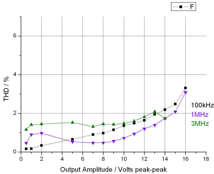
fig. A9: Non-linearity at high output levels (total harmonic distortion, THD), 10Vpp version
