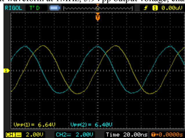
A2: Typical output waveform at 10MHz (Quad 1-10), 6.4Vpp output voltage , ch. B and C
