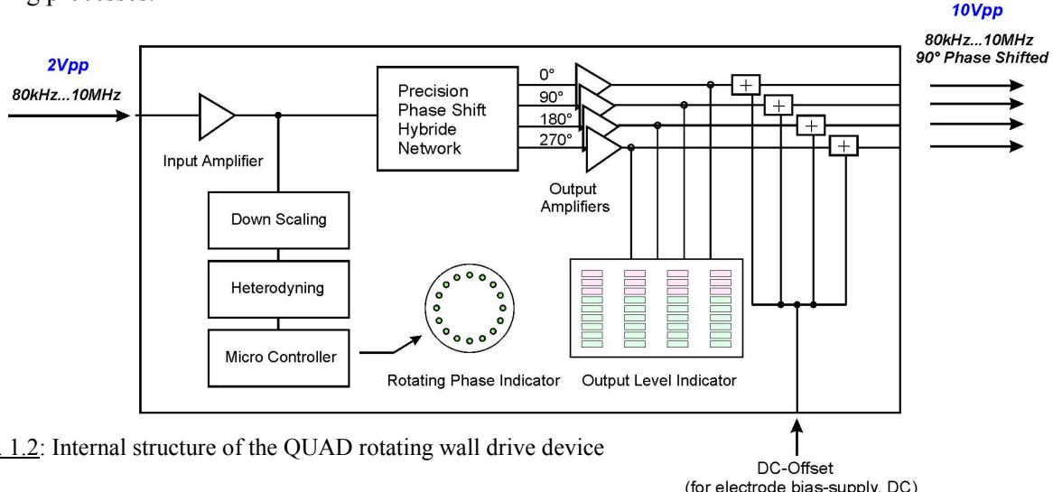
Fig. 1.2: Internal structure of the QUAD rotating wall drive device
