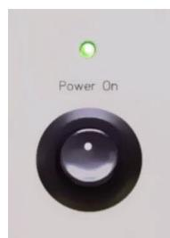
The device is powered up after turning on both the rear-side mains supply switch and also the power switch on the front plate. The Power-on-LED (green) indicates proper operation of the internal +30V supply circuitry.
