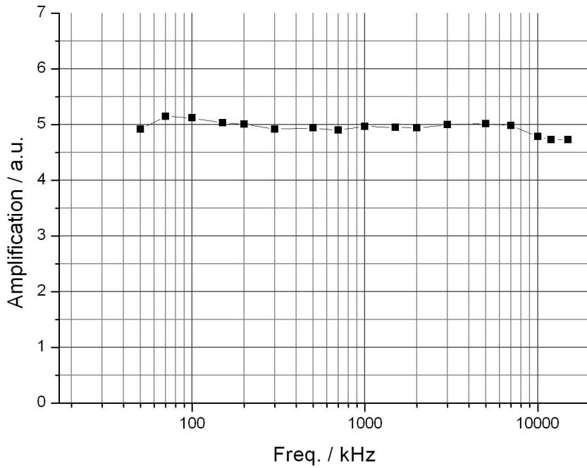
Fig. A8: Gain flatness vs. frequency
