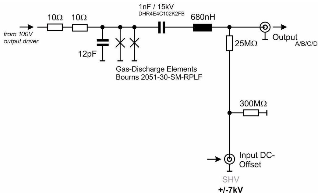
fig. A13: Circuit diagram of high voltage offset output stage  $\pm 7kV$  floating version. An external DC offset of up to  $\pm 7kV$  may be applied and is superposed to the AC signals from the internal phase shifter by means of a simple RC circuitry. Diagram shows one of four branches.
