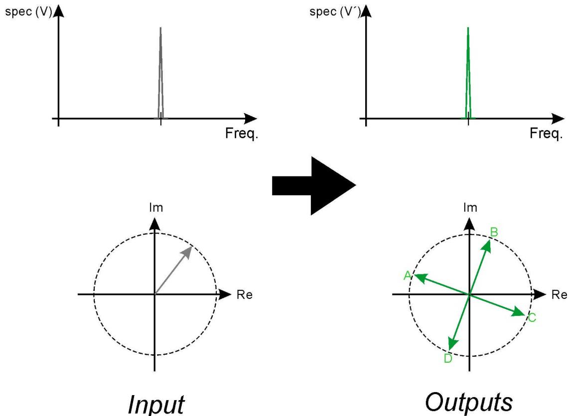
**Fig. 1.3:** Illustration of device functionality by comparing the input signal with the output signals. A sine wave with certain amplitude and frequency, fed in at the input, is converted into four 90° phase-shifted signals at the four outputs A-B-C-D. A constant phase relation of 90° and equal amplitude of the four output signals is maintained over a wide frequency range.
