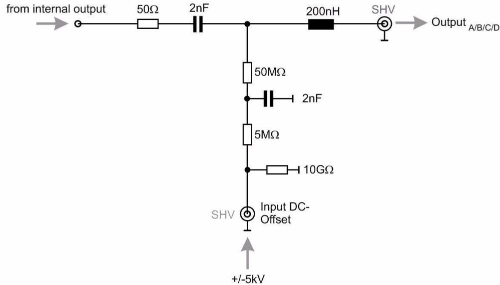
fig. A12: Circuit diagram of high voltage offset output stage. An externally supplied DC offset of up to  $\pm 5kV$  (max. value depends on rating) is filtered by a  $5M\Omega \times 2nF$  low pass and subsequently superposed to the AC signals from the internal phase shifter. Diagram shows one of four branches.
