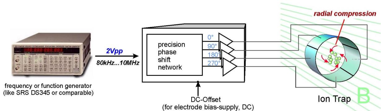
Fig. 1.1 Ion trap setup including a QUAD 1-5 rotating wall drive
