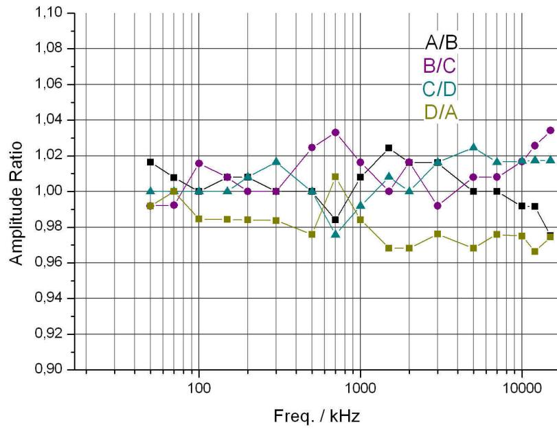
fig. A11: Typical amplitude mismatch vs. frequency
