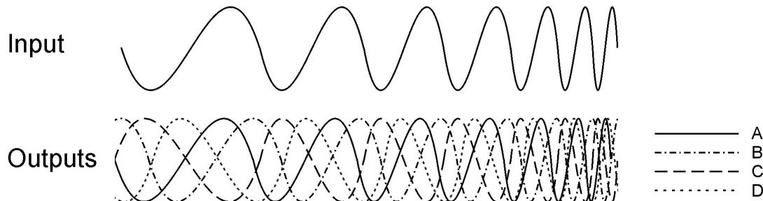
fig. 4.3 Example for a possible waveform; a swept sine wave may cover a broad frequency range in order to meet the plasma rotational frequencies, which might not be known precisely at the beginning. The sweep may be repeated several times to achieve the desired result of ion compression.
