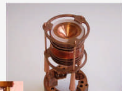
Trap for Ultrahigh Precision Mass Spectrometry, in Collabor. with GSI Darmstadt/ Univ. Mainz, Germany 2002 - 2006
